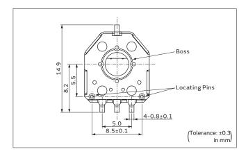
Determine the dimension of the locating holes as follows, depending upon the method of mounting the product (when mounting the product using a mounter or mounting it by hand).
